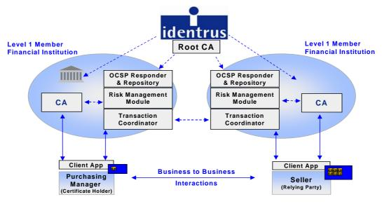
Figure 1: Functional architecture of Identrus system
